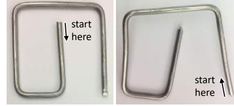
Fig. 5. We may fabricate this spiral-shaped wire (left) from inside to outside, but if we reverse the fabrication direction, the resulting wire (right) may become ill-shaped due to wire-machine collision.
